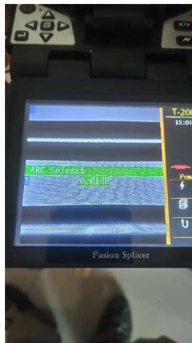
Lampiran 5. 6 Splicing fiber optic
